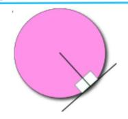
The angle between a tangent and radius is a right angle.
